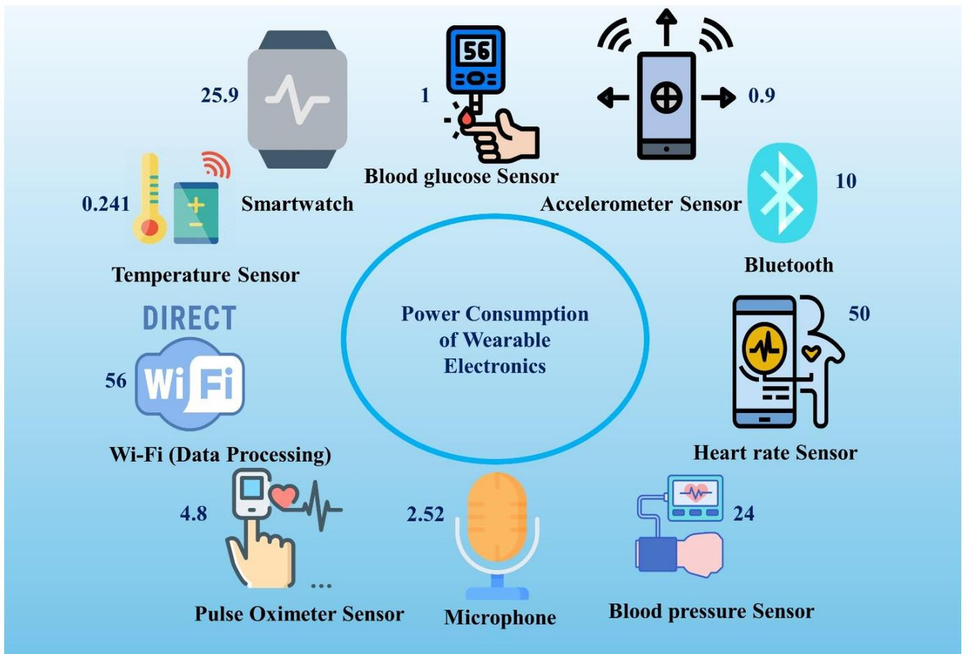
**Figure 14** Power consumption of wearable electronics (Numerical values are in mW).<sup>61,173,174</sup>
