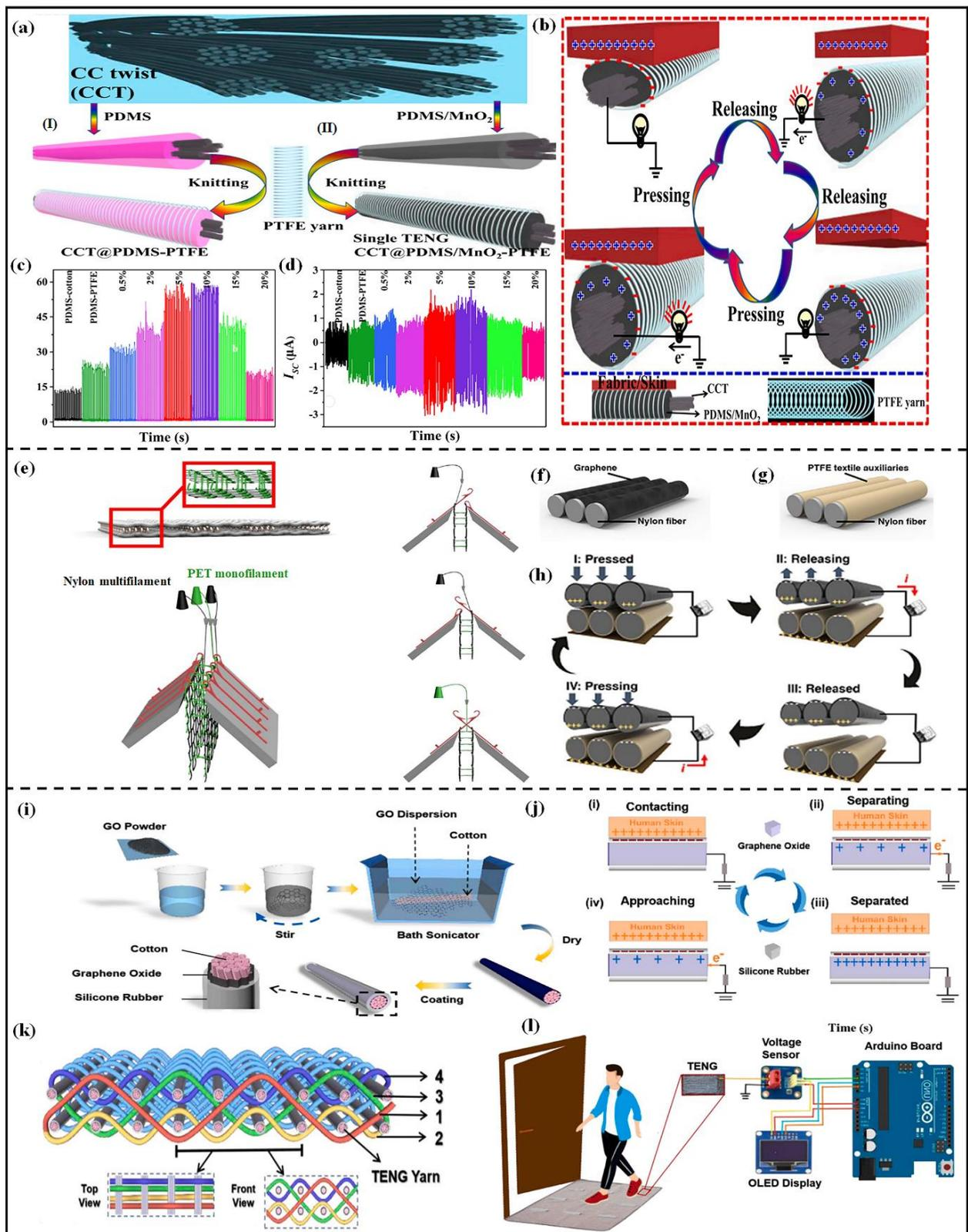
**Figure 9** 2D knitting based TENG (a) Schematic of the round-tripping knitting process for TENGs: a-i) PTFE yarn closing around pure CCT@PDMS and a-ii) CCT@PDMS/MnO<sub>2</sub>NW elastic yarns, (b) Schematic illustrations of the working mechanism of the T-TENG, (c) output voltage and (d) output current of TENGs. Reproduced with permission: Copyright 2021,
