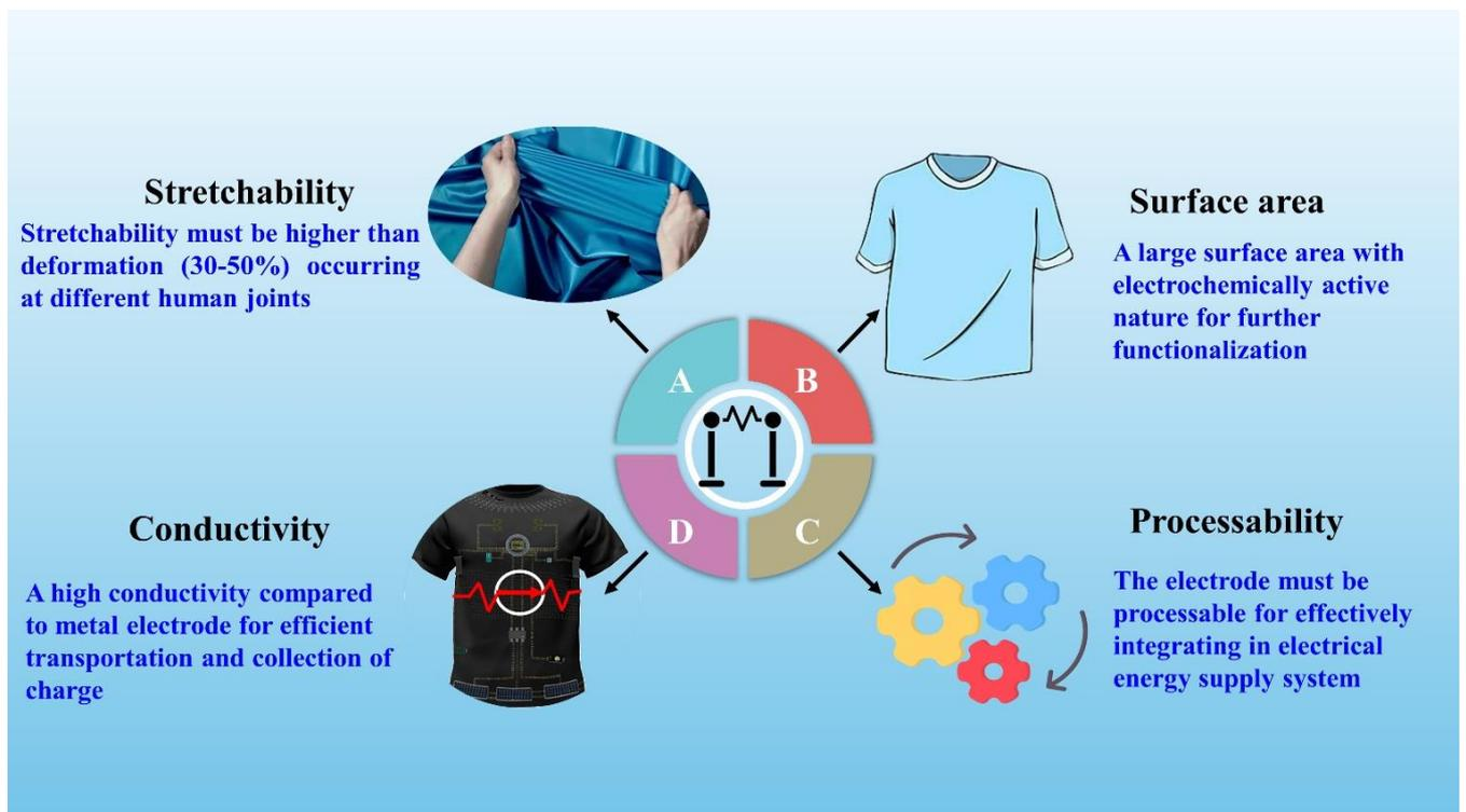
**Figure 5** Key factors of an ideal wearable electrode.<sup>114</sup>
