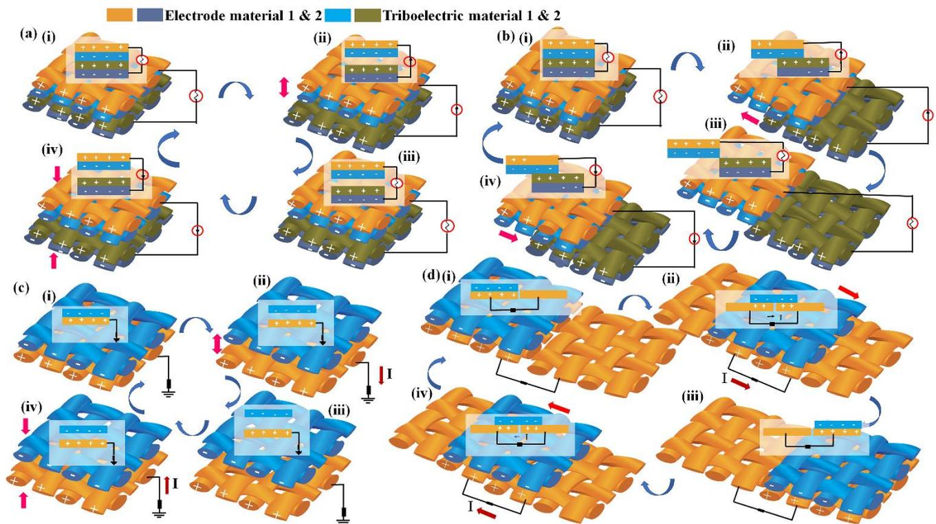
**Figure 2** Four fundamental operational modes of textile-based TENGs, including (a) contact-separation mode, (b) lateral sliding mode, (c) single electrode mode, and (d) freestanding triboelectric mode (Explained in clockwise direction).
