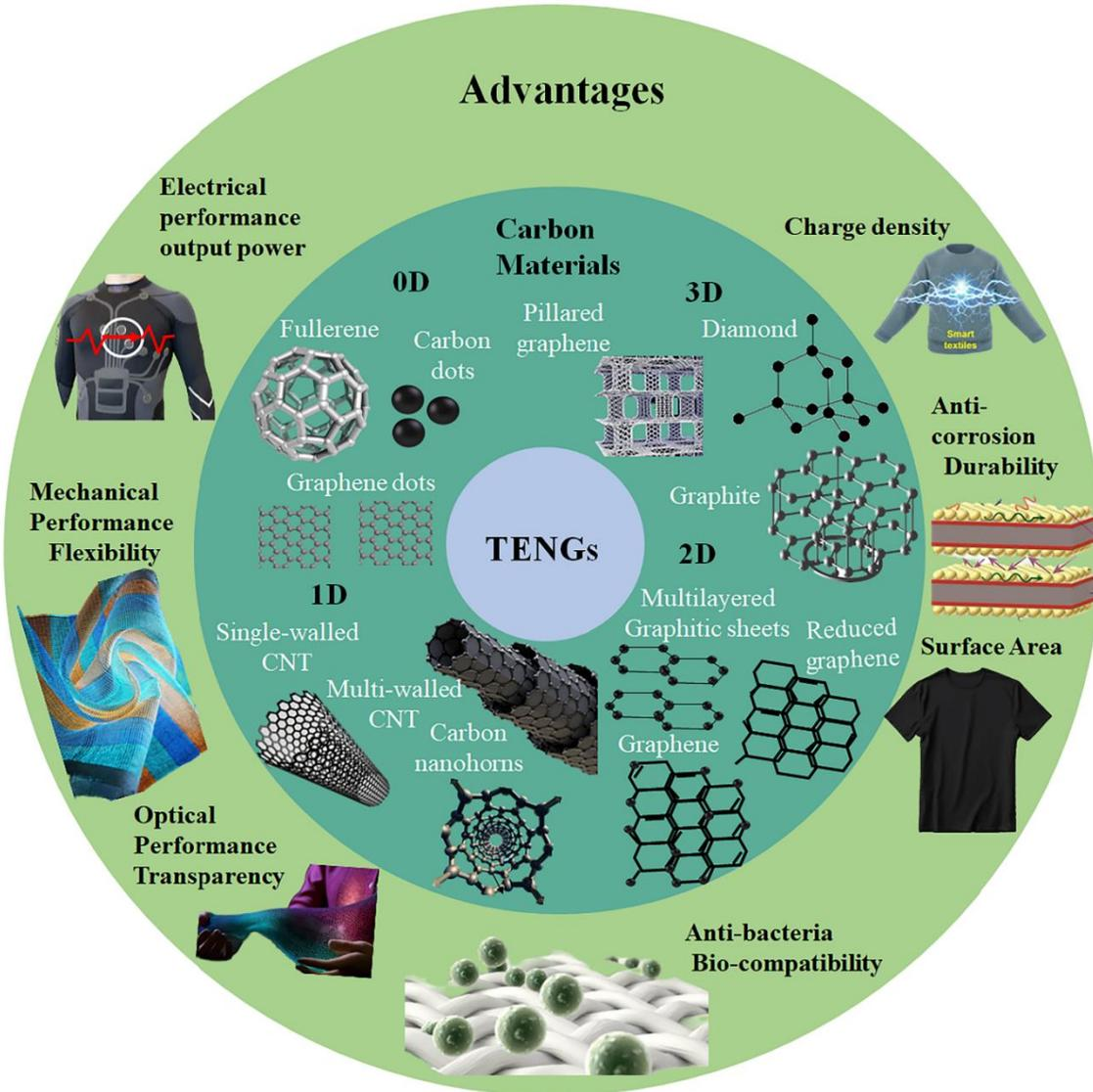
**Figure 4** Different Low-dimensional carbon nanoparticles for T-TENG and their advantages.<sup>23</sup>
