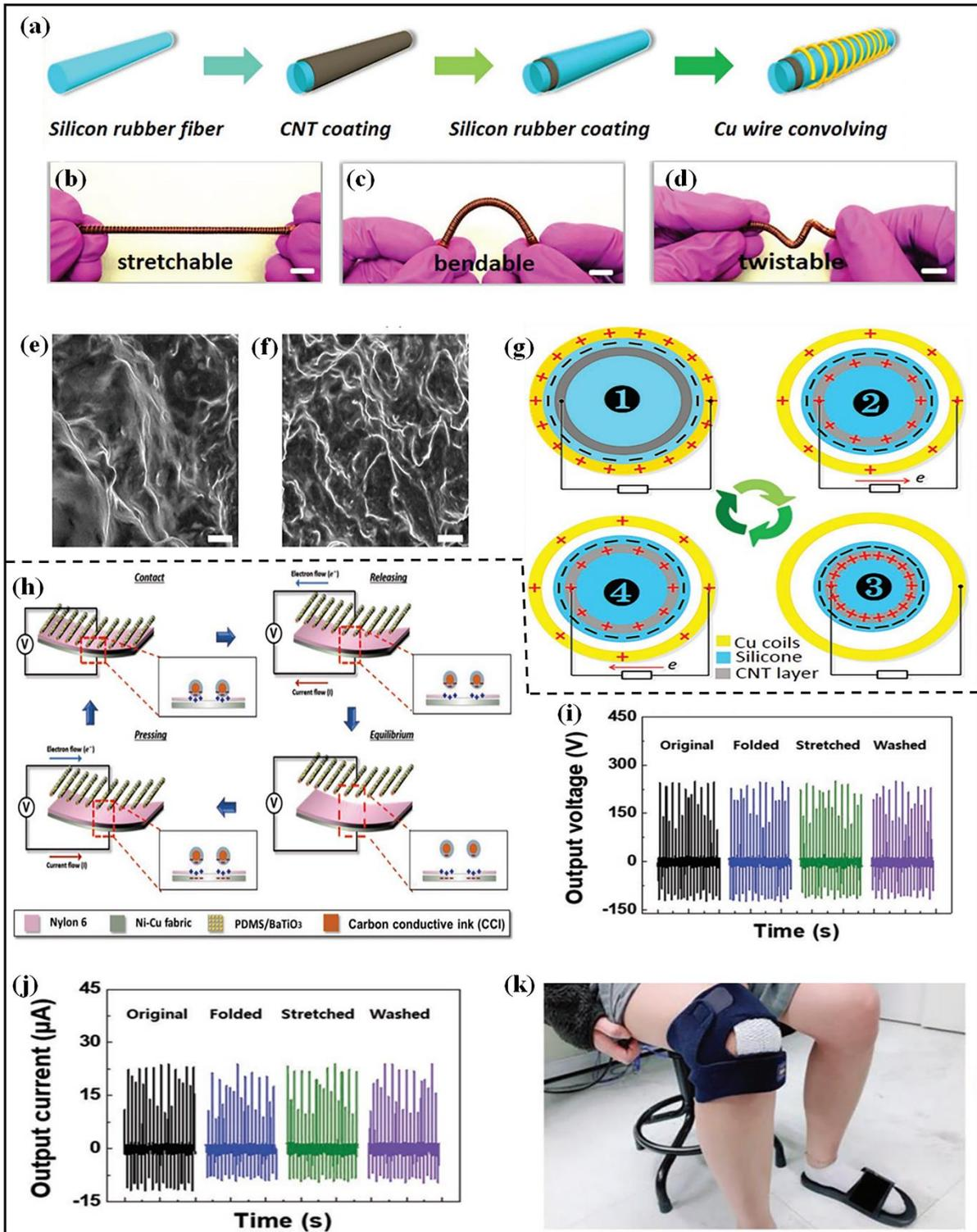
**Figure 13** The structure schematic of silicone rubber, CNT and copper wires based elastomeric fiber-like TENG. (a) Fabrication process of the fiber-like TENG, the digital images of the fiber-like TENG at different states, (b) stretched state, (c) bent state, and (d) twisted state, Zoomed-in
